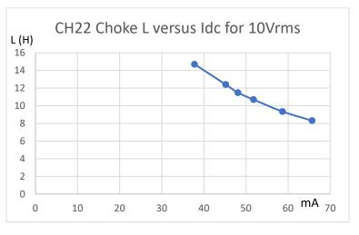
As an independent test, an LCR meter (MCP BR2822) measured the Rola choke as 11.8H with 0.21Vrms 100Hz excitation and no DC current.
