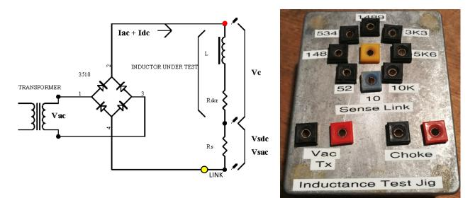
Three meter measurements are needed for each calculation of choke inductance:
